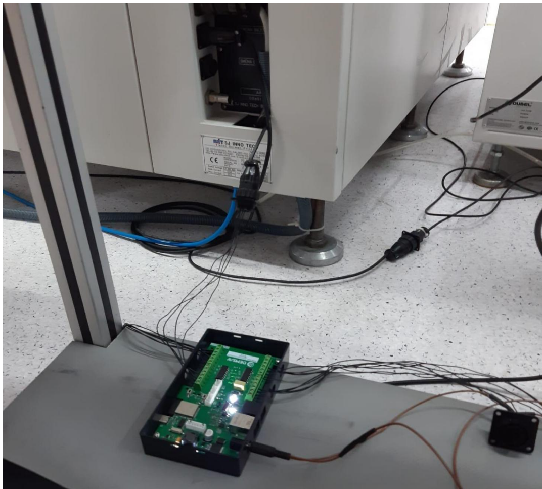
Figure 6. Physical integration of the IoT module into SMT machines and SMEMA signal lines.
