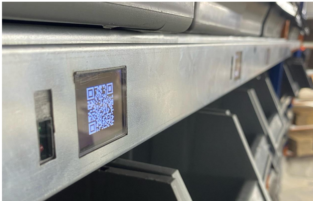
Figure 3: Display of dynamic QR code on the digital label
