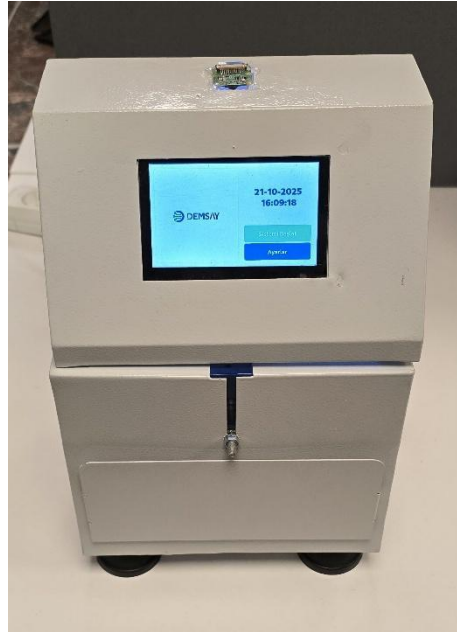
Figure 2: Physical implementation of the next-generation control and placement board.
